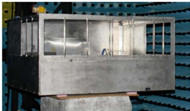
FIG. 1. Metallic enclosure used for the nonlinear time-reversal experiment in an anechoic chamber. The nonlinear element is placed inside the enclosure while transmit and receive (TRM) antennas are placed outside the enclosure.
